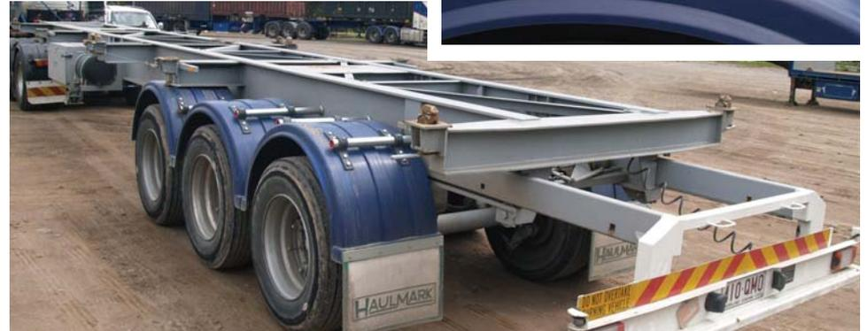
Air operated locking pins and no maintenance sliding suspension mechanism provide a hassle-free operation.
