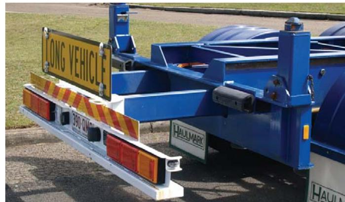
The pull out rear trailer concept provides greater versatility and on-road safety for the cartage of 14.6m (48 foot) containers
